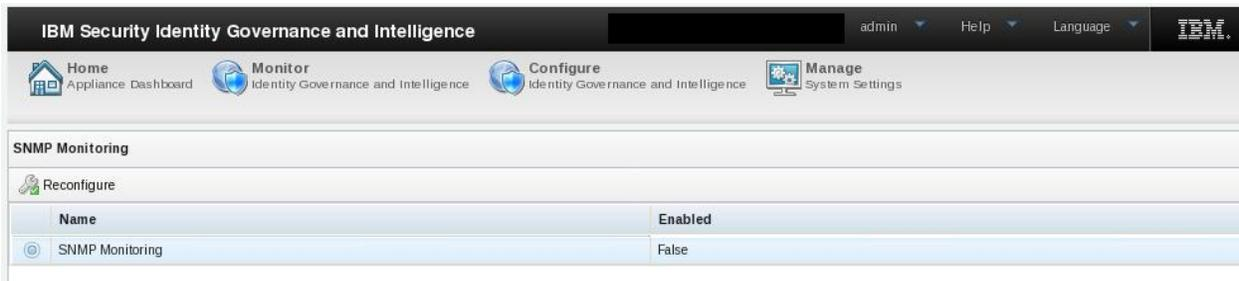
Figure 16: Enable Monitoring
